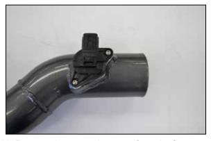
10. Remove the mass air sensor from the factory air filter housing and the install it into the AEM® intake tube and secure with the provided hardware
