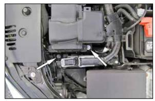
4. Remove the two bolts that secure the air filter housing to the vehicle.
